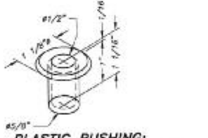
PLASTIC BUSHING: DETAIL 1 (ISOMETRIC) SCALE: 1" = 1"
